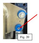
24. Next, mount the heat exchanger into the existing lower two holes in the radiator support with only the top bolts (make sure the inlet and outlet go behind the radiator support while installing the heat exchanger). Place the .20" thick spacers between the radiator support and the rubber grommets on the heat exchanger. Tighten the heat exchanger into place (Fig. 21-23).
